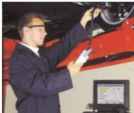
Ride Height measurements are taken with a Mercedes-Benz Electronic Level Gauge (available from MBUSA) and downloaded into the aligner through the built-in serial interface.
