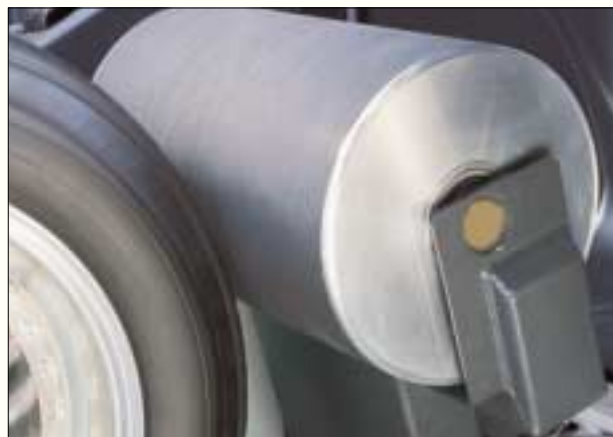
The load roller exerts up to 1,400 pounds of pressure against the tire assembly to detect non-balance, radial force-related vibration.
